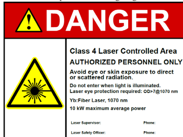
Sample ANSI Z535.2 Compliant Danger Sign for Class 4 Laser Areas
